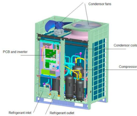
Figure 1. Internal view of the outer part of the variable refrigerant flow
